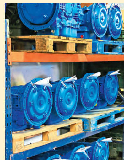
Before and after - Allison AT545 units as received and following remanufacturing. Clive notes that the external appearance of a received unit may not be an indicator of its internal condition
